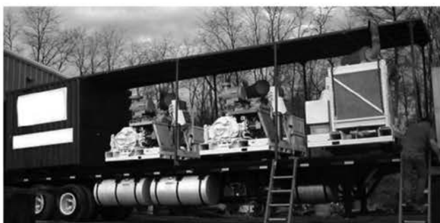
Fig. 4—Hydrodemolition pump trailer.
