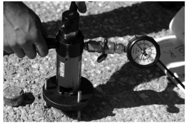
Fig. 8—Tensile bond test on prepared substrate.
