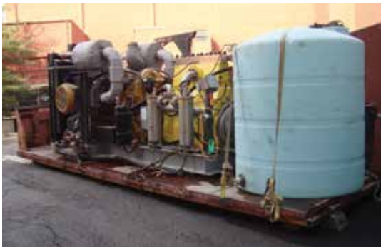
Fig. 5: Single unit small hydrodemolition pump set-up
