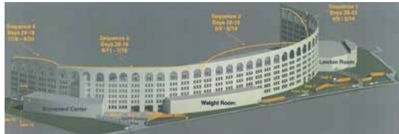
Fig. 3: Bay sequencing at north end of structure
