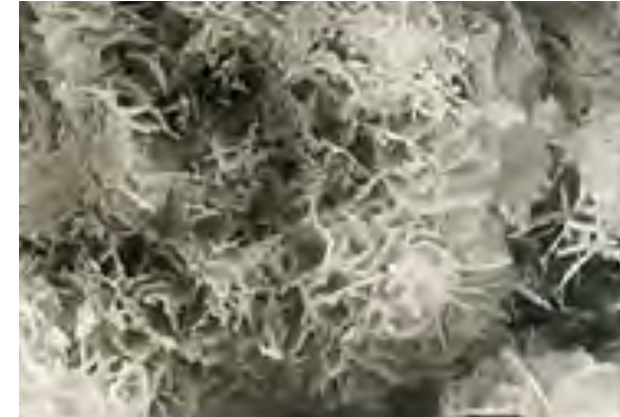
MICROPHOTOGRAPH: PORTLAND CEMENT IN EARLY STAGE OF HYDRATION
