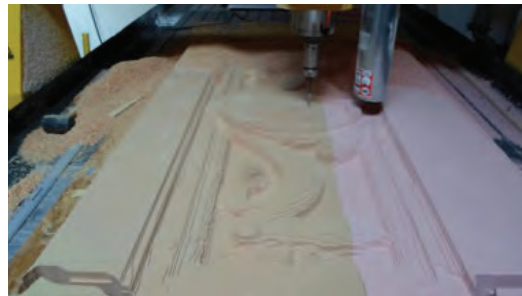
Fig. 9: Fabricating foam panel using CNC mill
