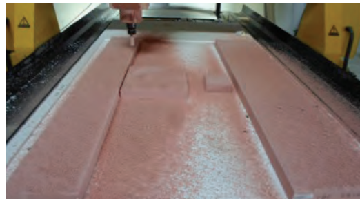
Fig. 8: Beginning of foam milling process
