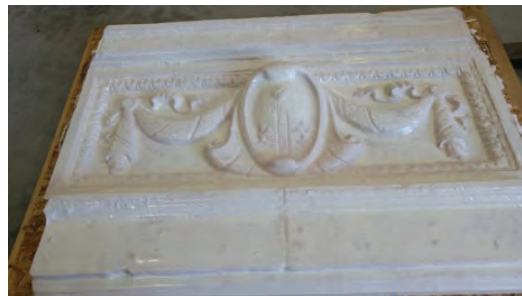
Fig. 11: Foam panel master copy coated with polyurethane
