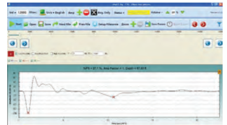
FTG Software Showing Sonic Echo Depth Measurement
