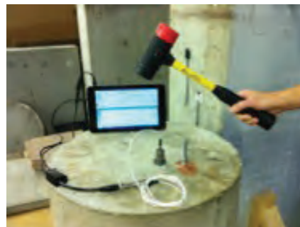
FTG-1 System shown with Data Acquisition Platform (Tablet not Included)
