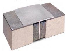
Self-expanding, precompressed foam, plus silicone, provides the noninvasive anchoring for QuickCover
