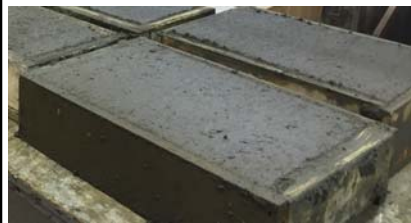
Composite specimen after spraying and screeding
