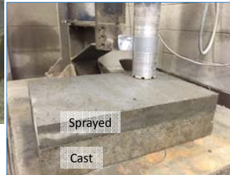
Composite specimen after spraying and screeding
