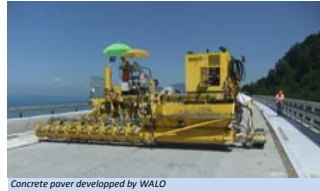
Concrete paver developed by WALO
