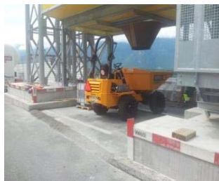
Motorized buggies to bring material in front of the paver
