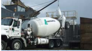
Loading and batching in ready-mix truck at Lafarge plant
