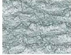
CSP 9 (heavy scarification)
