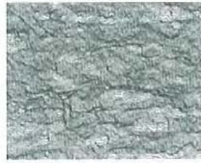
CSP 6 (medium scarification)
