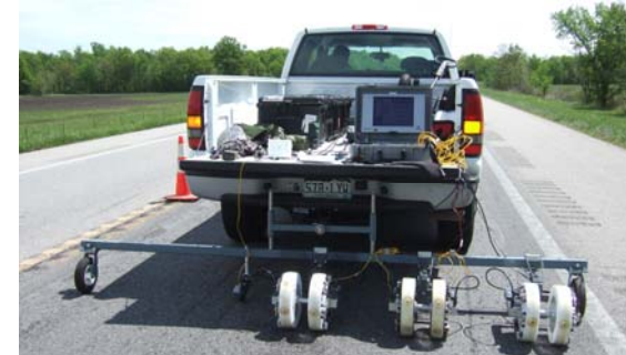
Prototype Pavement Scanner on Kansas Asphalt Pavement site with 3 pairs of wheels spaced 150 mm (0.5 ft) apart for combined Impact Echo and Spectral Analysis of Surface Waves scanning.
