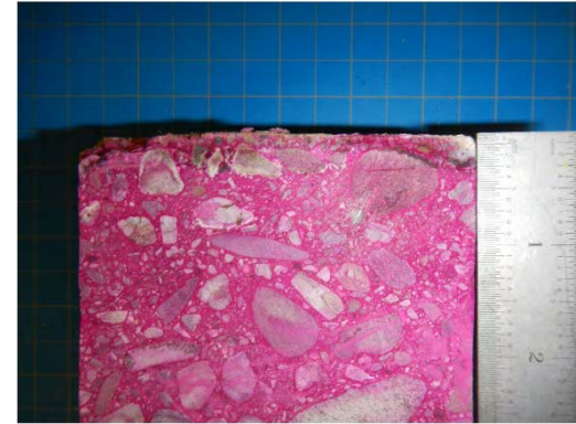
Photo #1– Depth of carbonation on sample P109G-B
