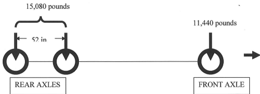
Fig. 2 a. EMPTY TRUCK - LOAD ON AXLES
