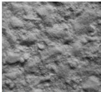
Fig. 6.7: CSP 7 (heavy abrasive blast)
