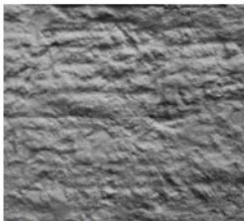
Fig. 6.6: CSP 6 (medium scarification)
