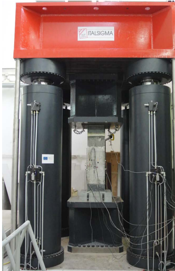
Mega testing machine (30.000 kN, 3000 tons axial capacity)
