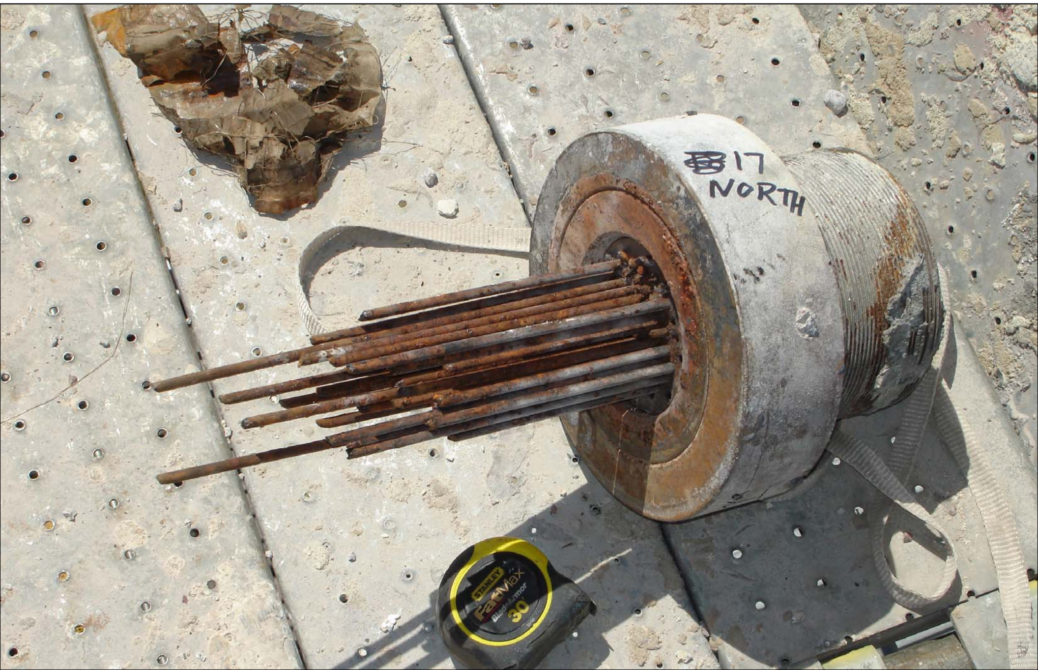
Failed end anchorage of post-tensioned cable. Failure caused by Hydrogen Embrittlement. Post-tensioned force 420,000 pounds.
