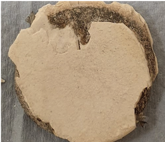
Fig. 8: Zinc corrosion byproduct surrounding core from galvanic anode removed after 20 years in service
