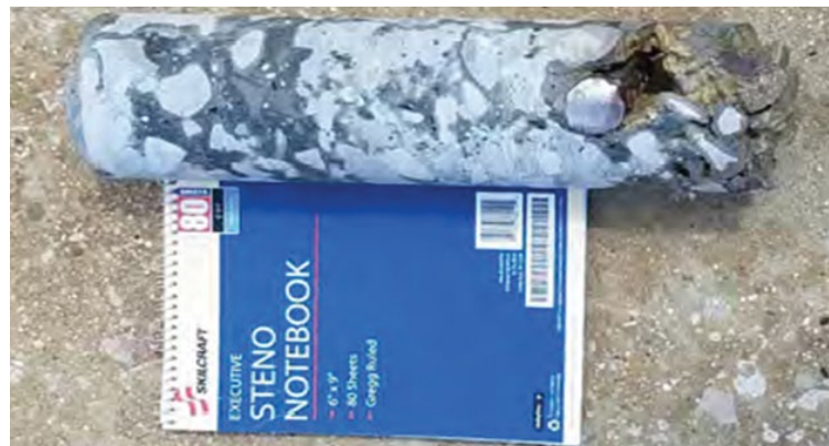
Fig. 8: Core 5—Partially Filled Core, left dark areas filled with epoxy and right area (bottom of core) partially filled
