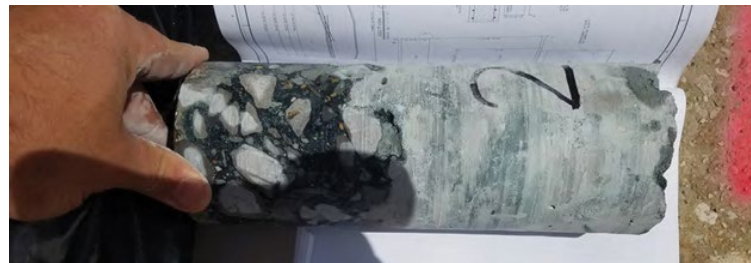
Fig. 6: Core 2—Darker, black section is filled with epoxy resin
