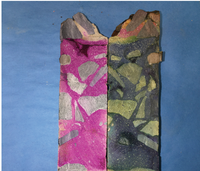
Fig. 9b: Carbonation—core treated with both phenolphthalein and rainbow indicator to show pH range through carbonation front
