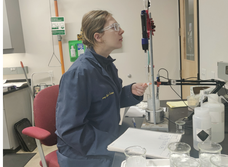
Fig. 10: Titration of powder sample for chloride concentration evaluation
