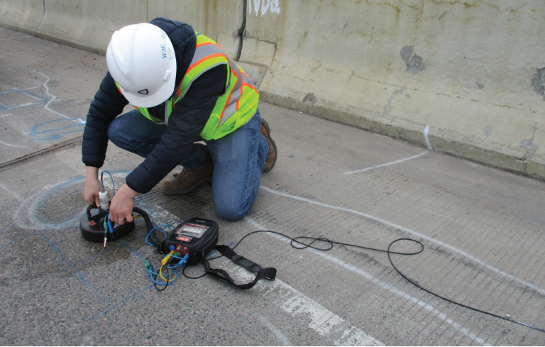
Fig. 6: Corrosion rate measurements
