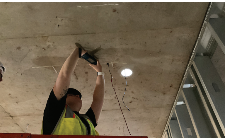
Fig. 7: Surface resistivity measurements
